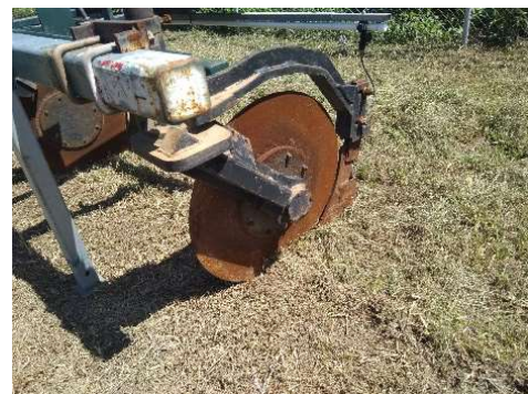
Photo 4 – Brew injection behind coulter
