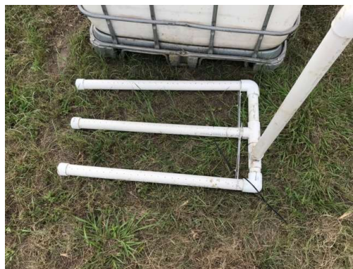
Photo 2 – Air spreader pipes
